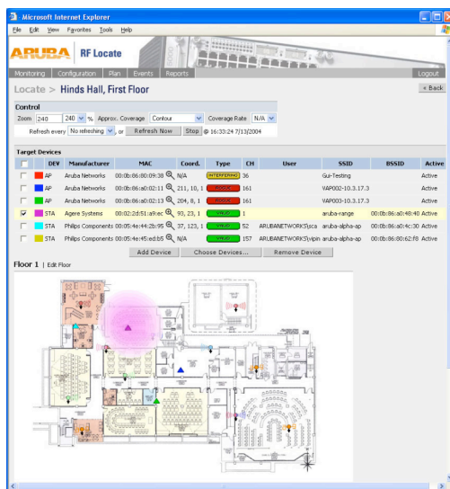
Figure 2 Multi-point triangulation pinpoints any 802.11 device
